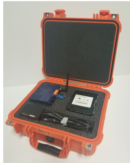
AdEdge’s 911 Box can be sent for on-the-fly changes and updates to PLC programs.
